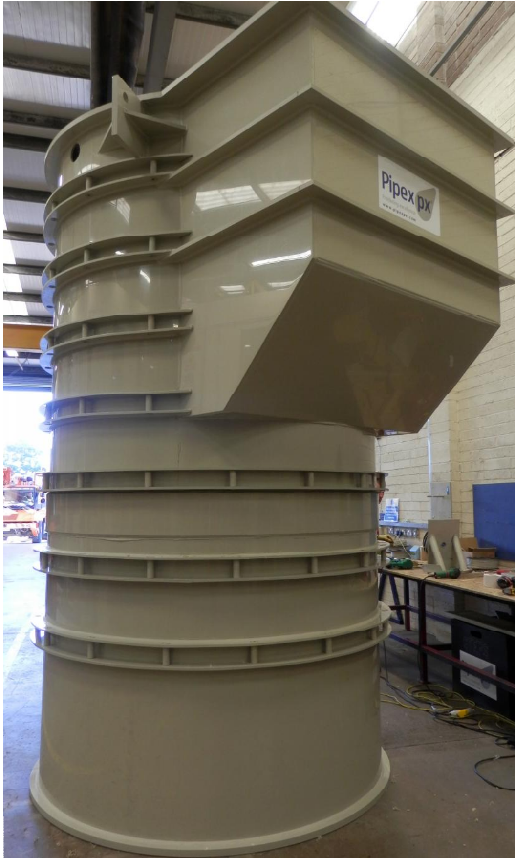
Bespoke Pumping Station manufactured from Advanced Thermoplastics
