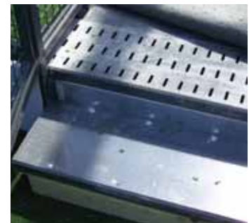
SAFPLANK® is offered in a slotted version to facilitate drainage like shown here on a Philadelphia Eagles stadium deck. Slots are placed in a longitudinal or transverse direction to the plank support to meet ADA standards.
